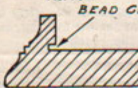
Bead cut made for rib strip with Bead Saw No. 1
